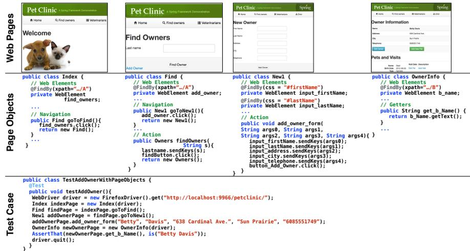
Fig. 2. Page objects generated by APOGEN to support a web test case development
