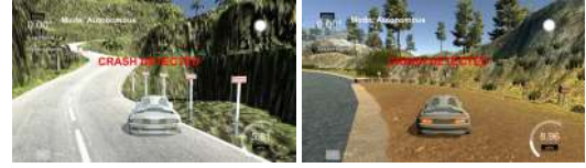
Figure 6: Simulator crash/OBE detection.
