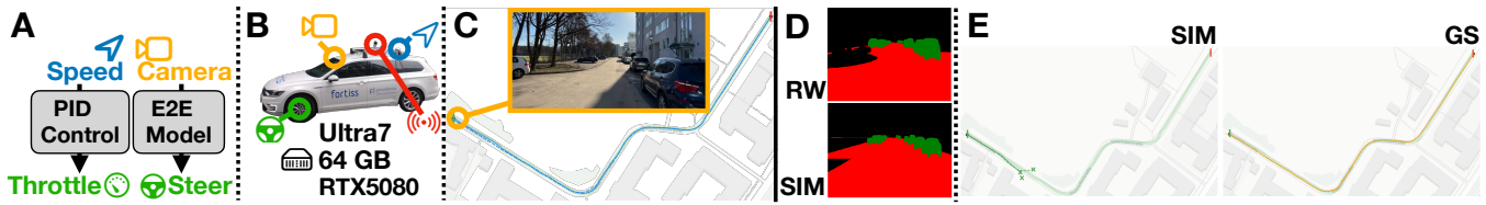
Figure 2: Validation setup and results: (A) the ADS, (B) the autonomous-driving platform used to collect the target recording, (C) the real-world collection scenario, (D) results of Scenario Reconstruction, and (E) Behavior Fidelity.
