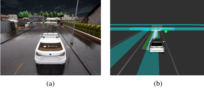
Fig. 1: Comparison of HiFi and LoFi simulations for an automated emergency braking scenario.
